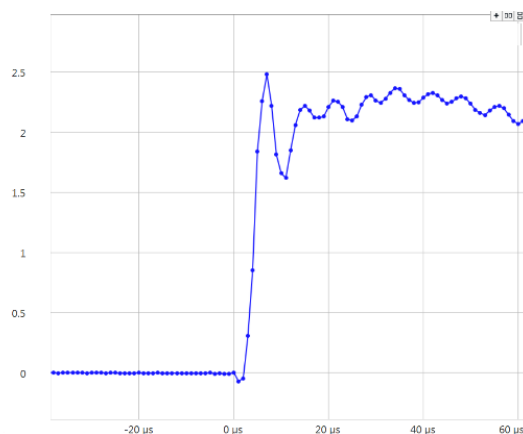
Fig. 1. Phase current of a field-recorded fault showing a 1 \text{ A}/\mu\text{s} slew rate.
