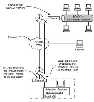
Fig. 1. Typical network topology with firewalls
