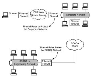
Fig. 7. Typical network topology with DMZ and firewalls
