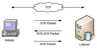
Fig. 3. TCP three-way handshake
