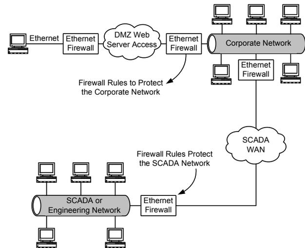
Fig. 7. Typical network topology with DMZ and firewalls
