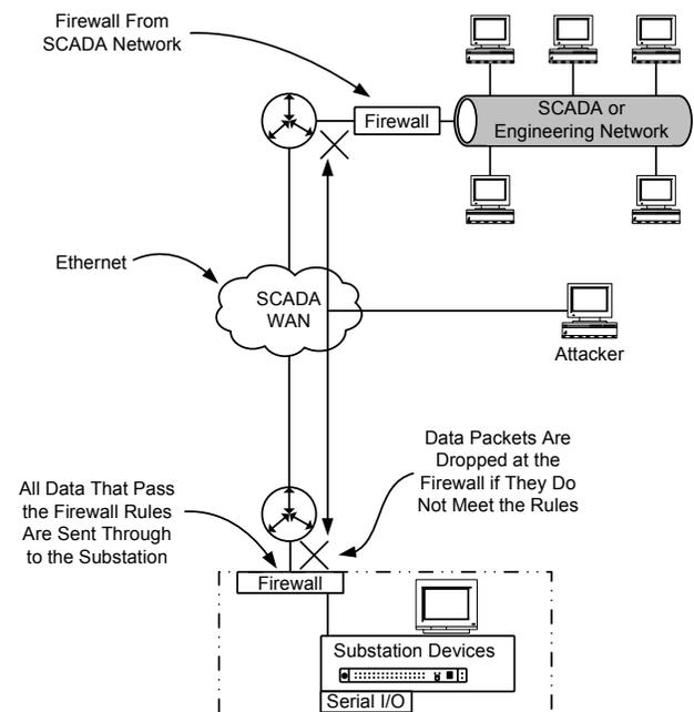
Fig. 1. Typical network topology with firewalls
