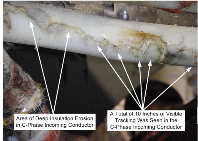
Fig. 31. C-phase incoming conductor damage
