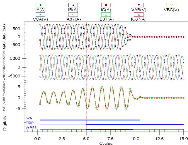
Fig. 9. Filtered event report of a differential trip
