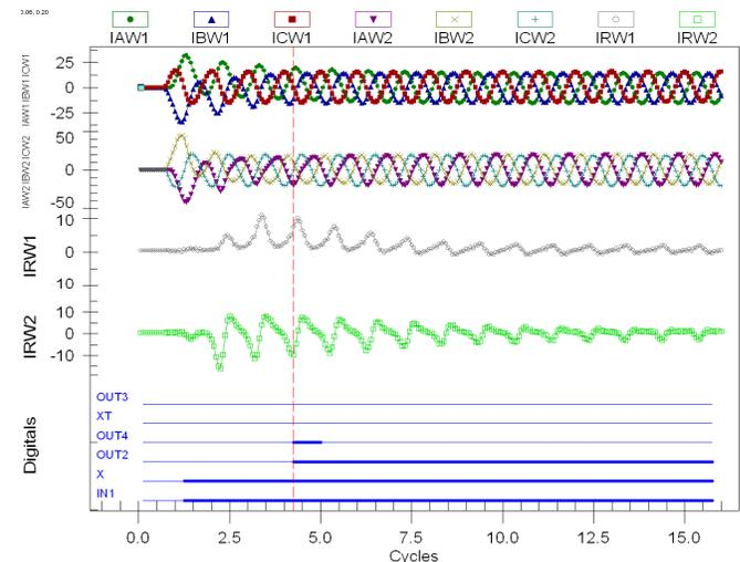
Fig. 14. Filtered event report of the phase differential trip
