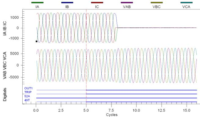
Fig. 1. Event report from a microprocessor-based relay showing a trip on thermal overload
