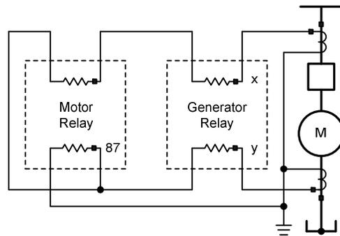
Fig. 21. 25,000 hp synchronous motor one-line diagram
