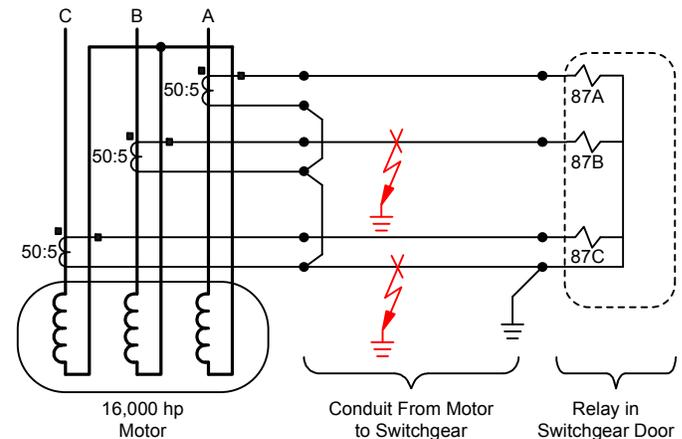
Fig. 11. Simplified three-line diagram with short-circuit locations shown
