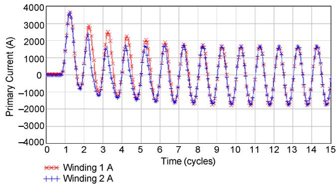
Fig. 15. A-phase Winding 1 and Winding 2 currents
