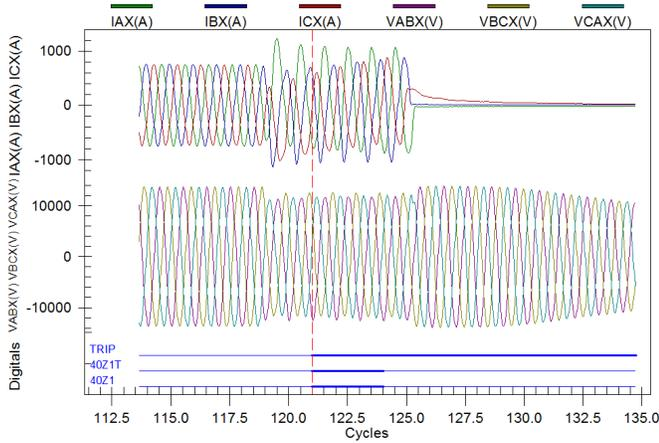
Fig. 22. Loss-of-field trip
