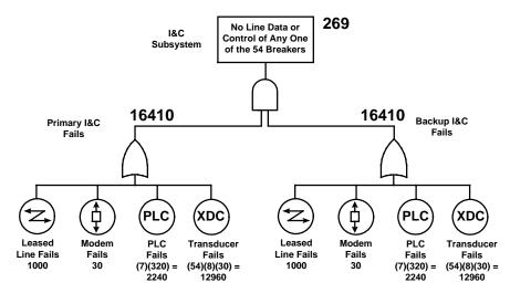
Figure 4: Fault Tree for PLC Centric Westmoreland I&C System
