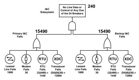
Figure 3: Fault Tree for RTU Centric Westmoreland I&C System
