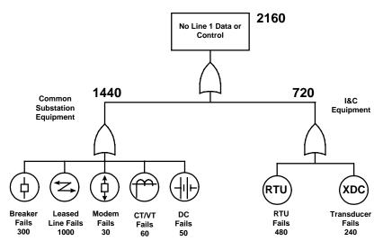
Figure 1: Fault Tree for RTU-Based I&C System
