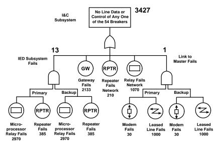
Figure 6: Multidrop Relay Network Centric Westmoreland I&C System
