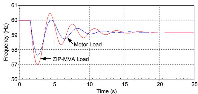
Fig. 2 Load Acceptance for Motor and ZIP-MVA Loads
