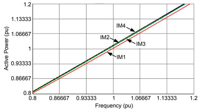
Fig. 7 Active Power Versus Frequency for Different IMs
