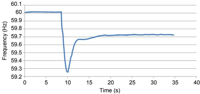
Fig. 5 Real Power Response for Load Acceptance Test From 4.7 MW to 6.9 MW
