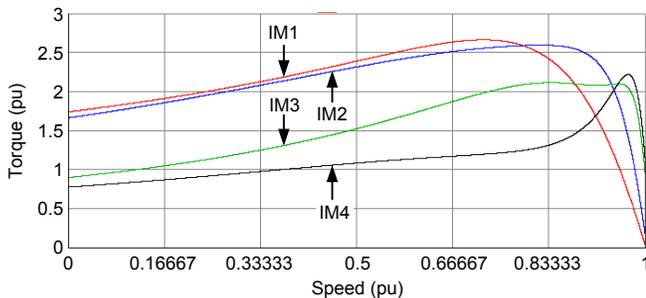
Fig. 6 IM Torque Versus Speed Characteristics
