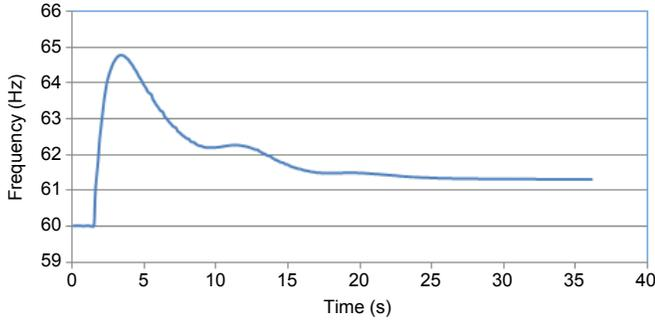
Fig. 3 Field Test Frequency Response for Load Rejection of 10.0 MW to 0 MW
