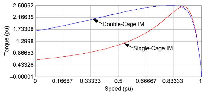
Fig. 8 Comparison of Single-Cage IM and Double-Cage IM Torque Versus Speed
