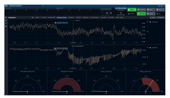
Example of Disturbance Detector Dashboard showing Forced Oscillation
