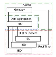
Fig. 1. Multilayer substation security approach
