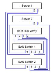
Fig. 2. Enterprise hardware redundant architecture
