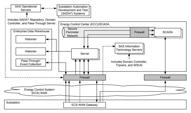
Fig. 7. SAS WAN and enterprise data flow diagram
