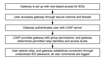
Fig. 6. Proxy remote access flow diagram
