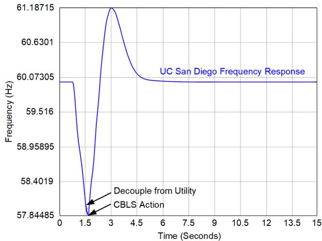
Fig. 12. Case A: Islanding for Grid Disturbance
