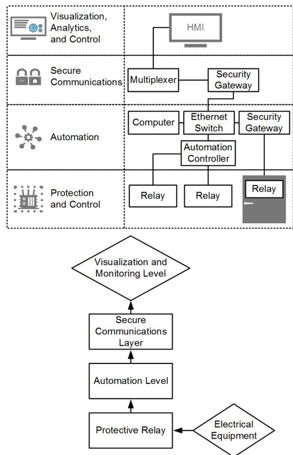
Fig. 13. Substation Automation and Control System
