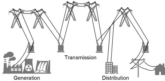
Fig. 1. Power System Diagram
