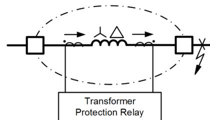
Fig. 9. Transformer Protection Relay Connection During External Fault
