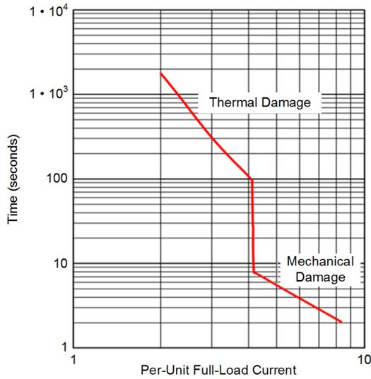
Fig. 10. Transformer Damage Curve [5]
