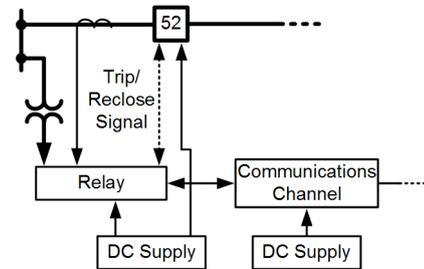
Fig. 3. Protection System Structure
