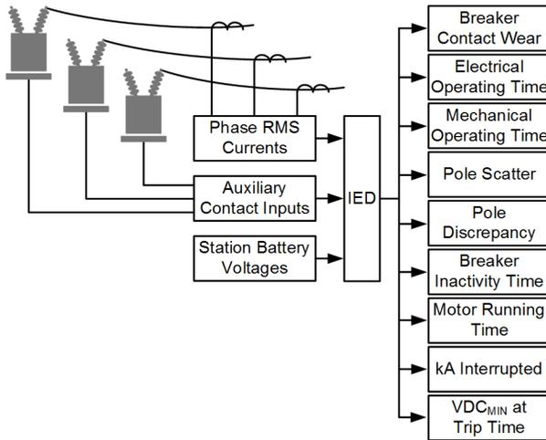
Fig. 4. Circuit Breaker Interface With Relays and Relay Monitoring Reports
