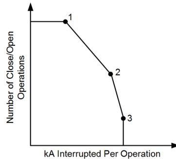
Fig. 6. Circuit Breaker Wear Contact Curve
