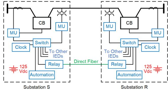
Fig. 6. System 2 Sampled Values Line Protection Substation Configuration
