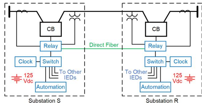
Fig. 3. System 1 Line Protection Substation Configuration
