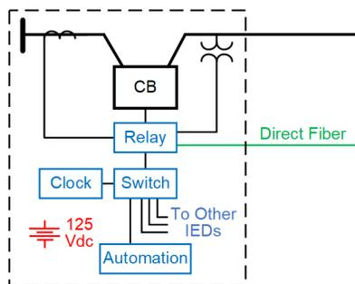
Fig. 1. Simplified Substation Protection, Automation, and Communications Diagram
