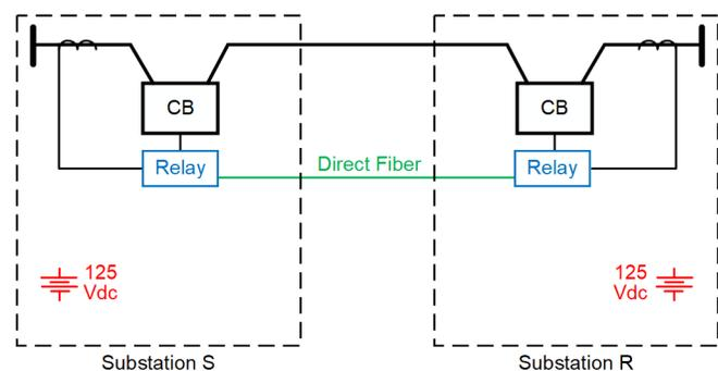
Fig. 4. Protection Elements Required to Detect and Clear a Fault
