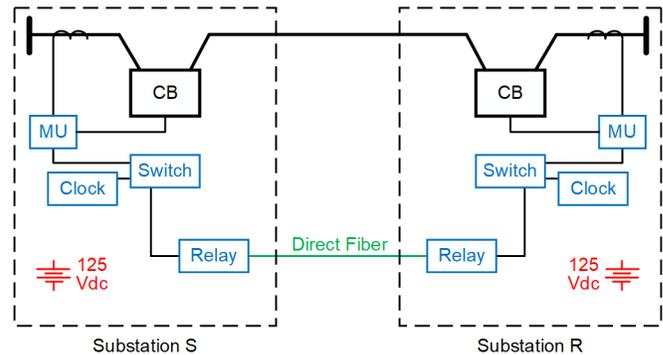
Fig. 7. System 2 Sampled Values Line Current Differential Protection Scheme
