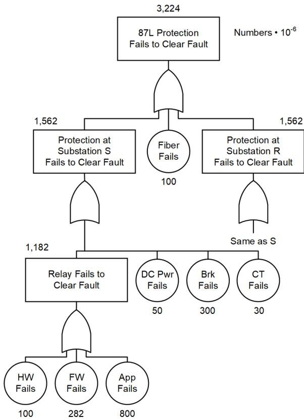
Fig. 5. System 1 Line Current Differential Protection Fault Tree Analysis
