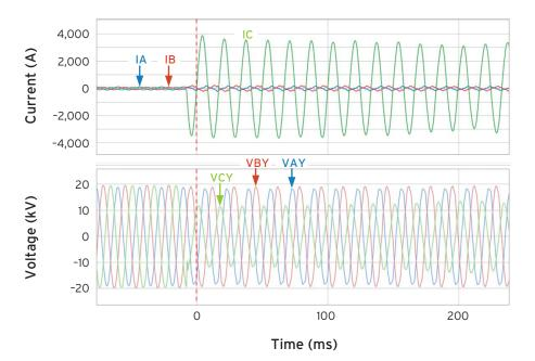
Figure 10—Oscillography from the SEL-651R showing the inception of a fault on Phase C.
