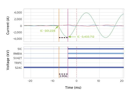
Figure 11—The assertion of the SEL-FT50 fault status Mirrored Bit from the SEL-FR12 approximately 4 ms after the fault inception.
