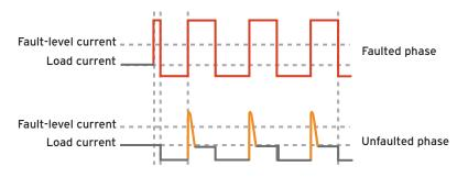
Figure 1—Simplified example of typical automatic reclose sequence.
