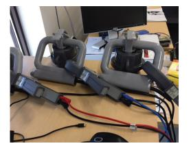
Figure 4—MCL120 current loops connected to SEL-FT50 transmitters in the test lab.
