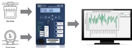
Figure 4—The SEL-735 Can Count Electrical Pulses for WAGES Monitoring
