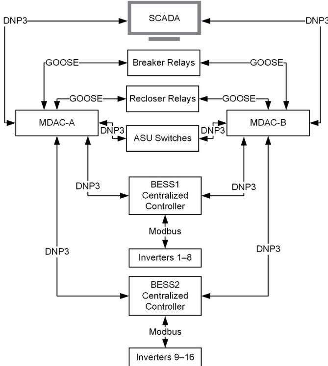
Fig. 4. BESS and distribution circuit data flow diagram
