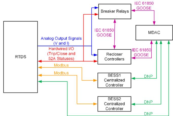
Fig. 13. Real Time Digital Simulator HIL setup
