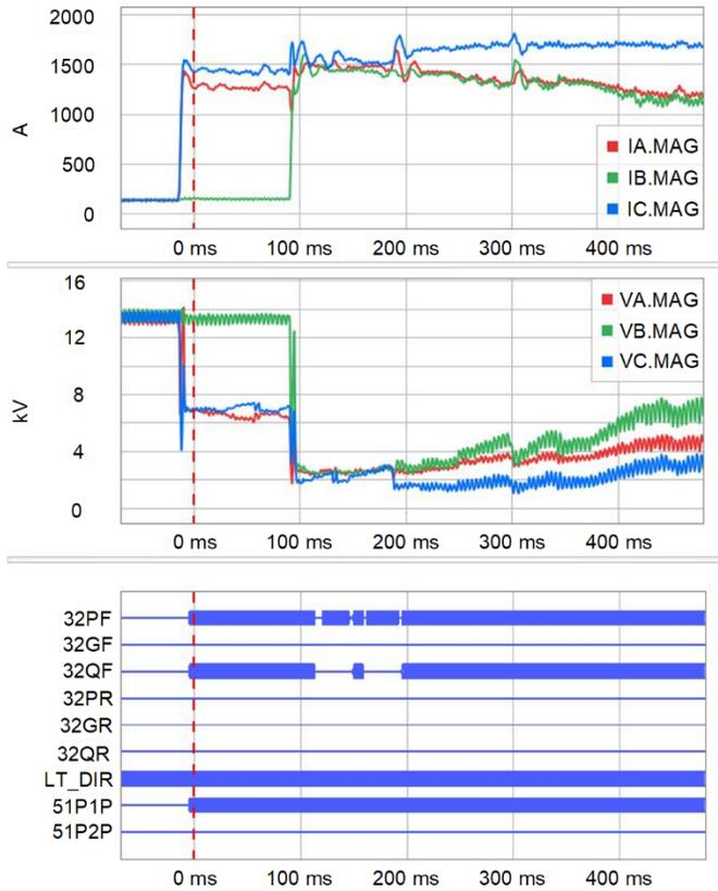
Fig. 10. Evolving fault at RCL6
