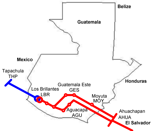
Fig. 2. The Guatemalan 230 kV network connects Mexico to the rest of Central America
