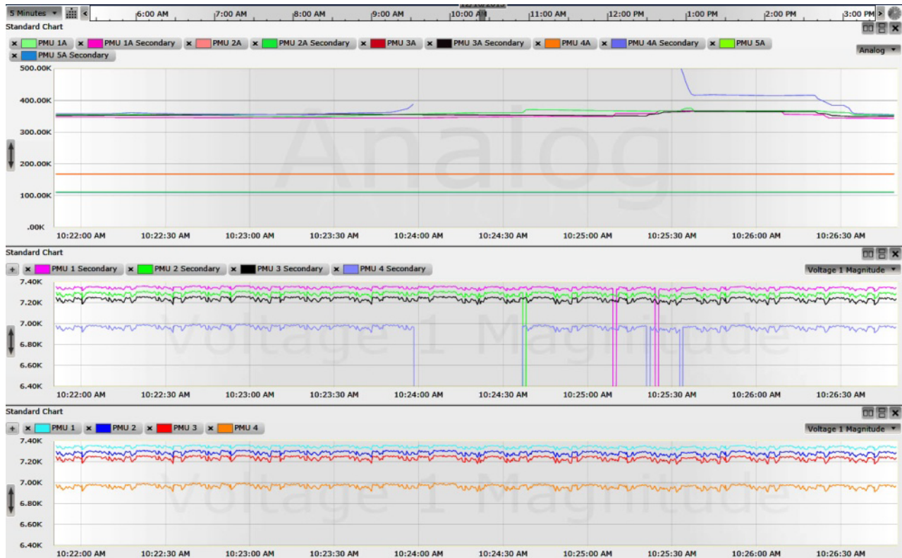
Fig. 4. PMU voltage magnitude V1 data plotted using serial radios (bottom) and cellular modems (middle) and the latency of each (top) over time.
