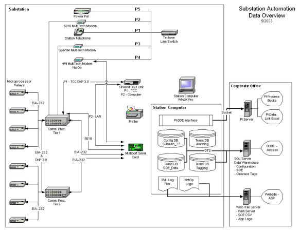
Figure 1 Substation Communications Hierarchy Overview
