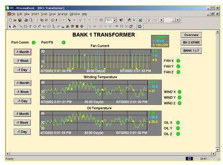
Figure 3 Monitoring Fan Operations Reduces Fan Failures
