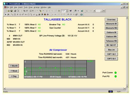
Figure 4 Breaker Air Compressor Monitoring Provides Early Warning of Impending Compressor Failures
