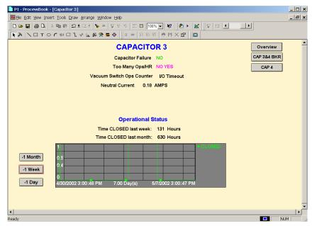
Figure 5 Typical Capacitor Operational Screen From a PI Database
