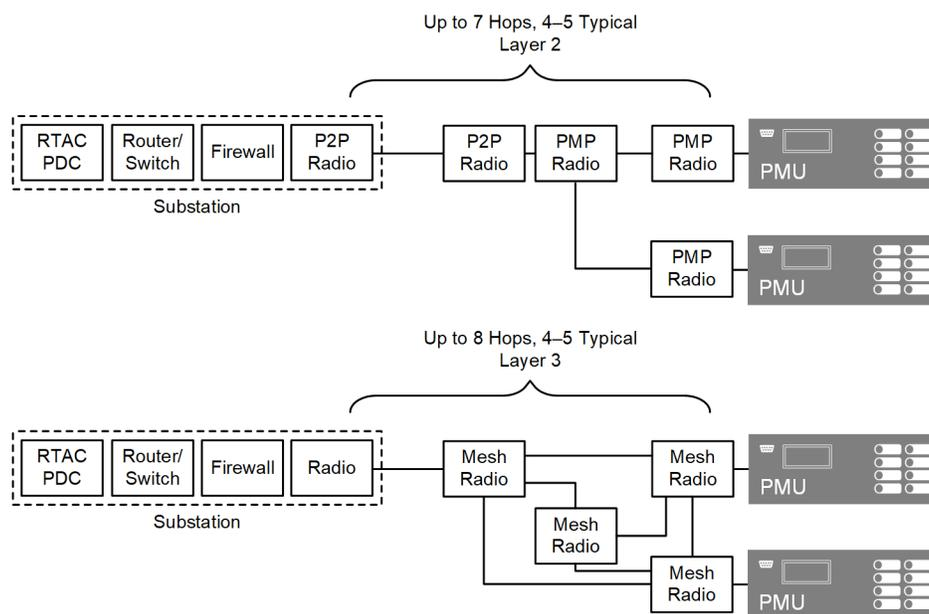
Fig. 7. P2P/PMP and mesh network solution architectures
