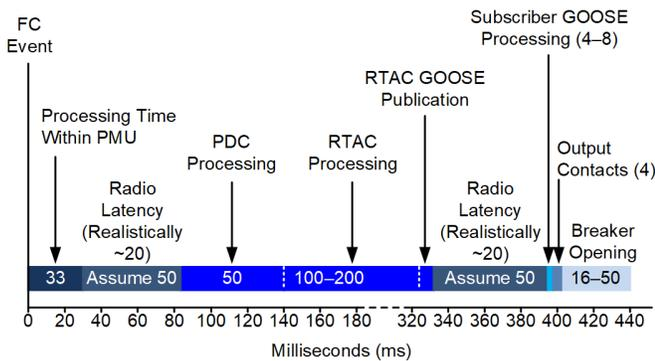
Fig. 16. FCP detection, processing, and isolation timing chart
