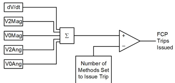
Fig. 4. Voting scheme for issuing GOOSE trip controls
