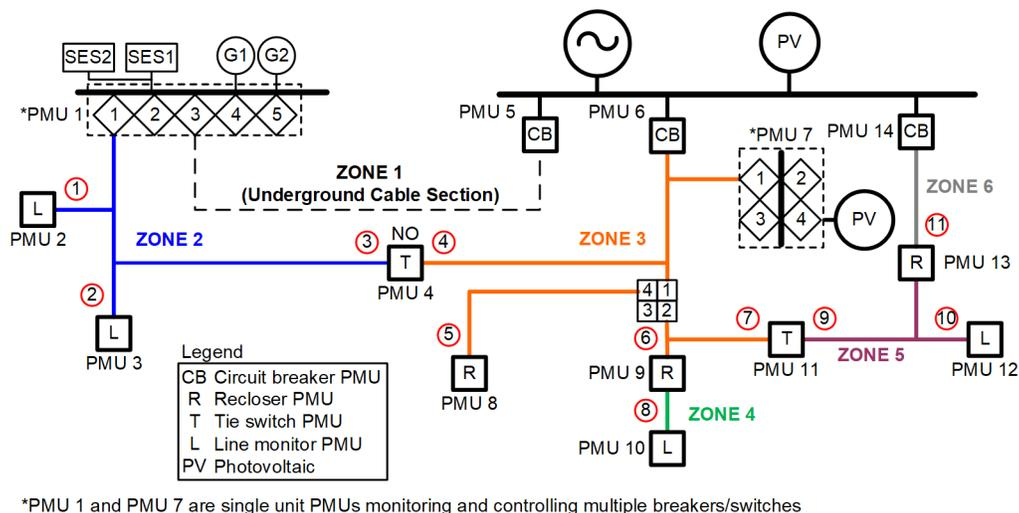
Fig. 9. SDG&E 12 kV rural distribution circuit
