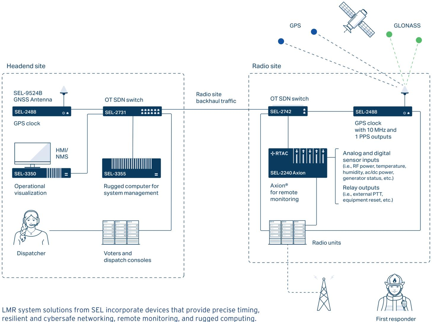
LMR system solutions from SEL incorporate devices that provide precise timing, resilient and cybersafe networking, remote monitoring, and rugged computing.
