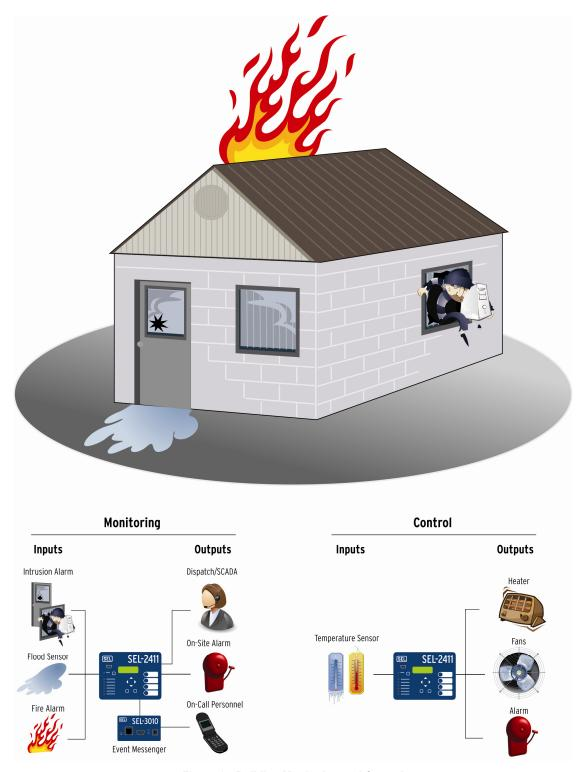
Figure 1 Building Monitoring and Control
