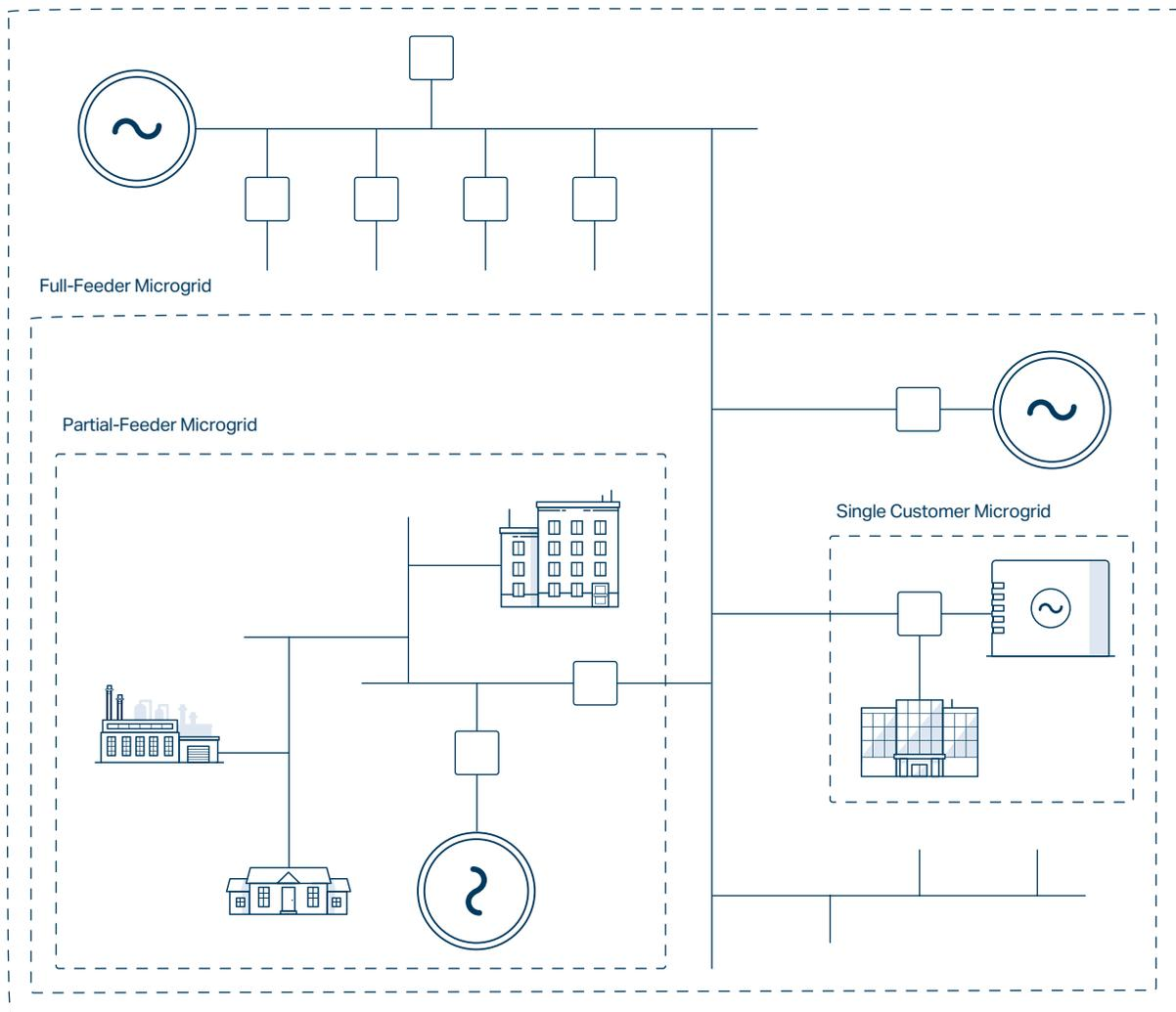
**Islanding Configuration Possibilities**—Within the microgrid, the SEL control allows one or more submicrogrids to operate, ensuring critical loads are always served.
