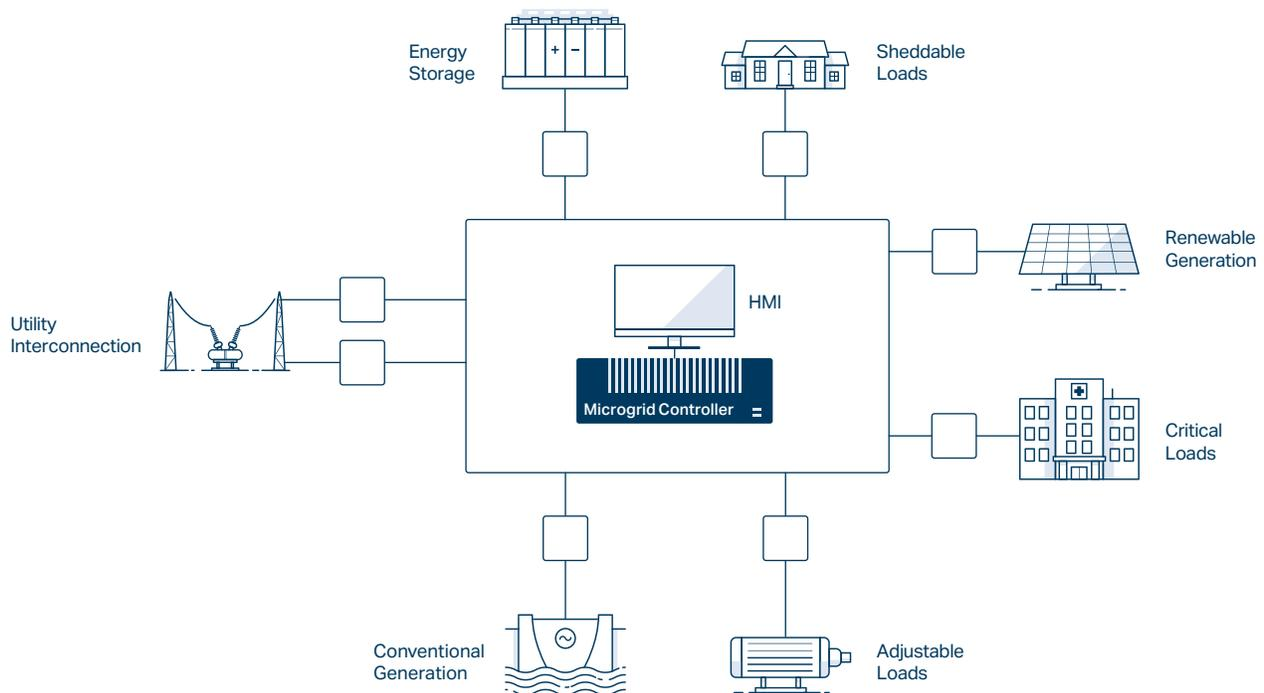
**Incorporate All Assets**—SEL microgrid control systems are capable of protecting and controlling many types of distributed energy resources.
