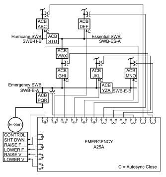
Fig. 6 Platform 2 Emergency Generator A25A
