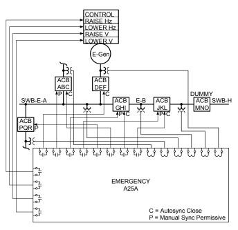
Fig. 3 Platform 1 Emergency Generator A25A
