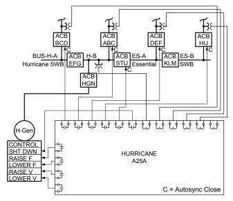
Fig. 5 Platform 1 Hurricane Generator A25A
