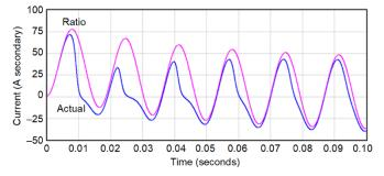
Fig. 18. Terminal CTs: CT2 Ratio and Actual Secondary Current
