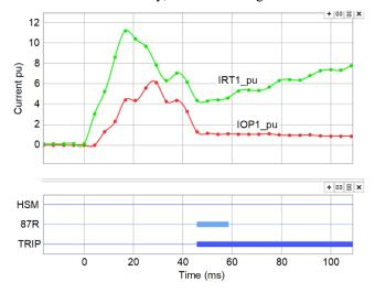
Fig. 21. External Single Line-to-Ground Fault With HSM Disabled
