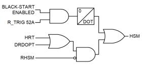
Fig. 7. HSM Enabled on Breaker Closing
