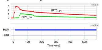
Fig. 24. Single Transformer Energization With HSM Enabled
