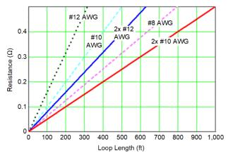
Fig. 4. Burden for Different Lead Lengths and Sizes
