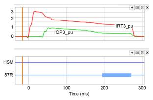
Fig. 23. Single Transformer Energization With HSM Disabled
