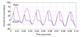
Fig. 17. Neutral CTs: CT1 Ratio and Actual Secondary Current
