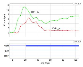
Fig. 22. External Single Line-to-Ground Fault With HSM Enabled
