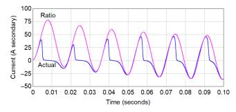
Fig. 3. Actual vs. Ratio (Ideal) CT Secondary Current
