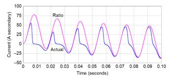
Fig. 26. CT1 Ratio and Actual Secondary Current With Parallel CT Leads
