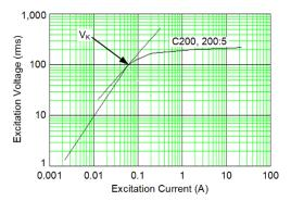
Fig. 2. Diagram of CT Excitation Characteristic [5]
