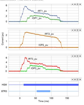
Fig. 25. Four Transformers Energized With HSM Enabled
