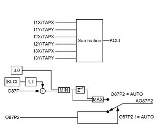
Fig. 11. Adaptive HSM Minimum Restraint Pickup Logic
