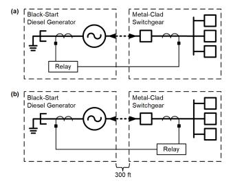
Fig. 15. Black-Start Generator Connected to Switchgear
