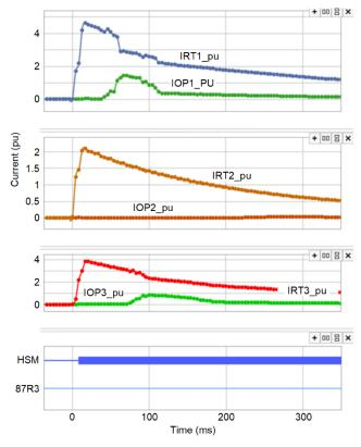
Fig. 27. Four Transformers Energized With Parallel Leads and HSM Enabled
