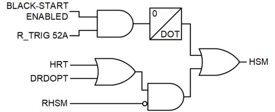
Fig. 7. HSM Enabled on Breaker Closing
