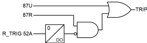
Fig. 13. Custom Blocking Logic for 87R Element
