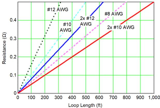
Fig. 4. Burden for Different Lead Lengths and Sizes
