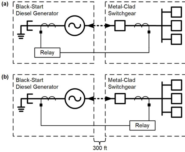
Fig. 15. Black-Start Generator Connected to Switchgear
