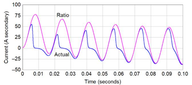
Fig. 26. CT1 Ratio and Actual Secondary Current With Parallel CT Leads
