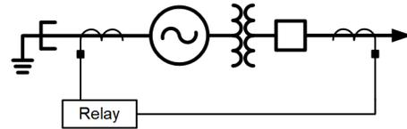
Fig. 12. Generator Differential With Transformer in Zone
