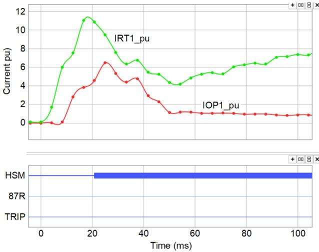
Fig. 22. External Single Line-to-Ground Fault With HSM Enabled
