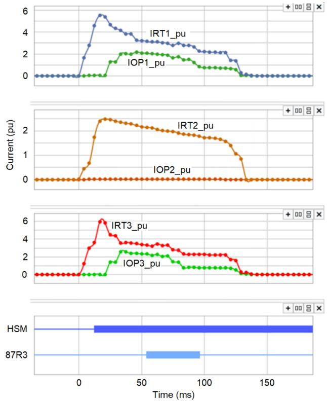
Fig. 25. Four Transformers Energized With HSM Enabled
