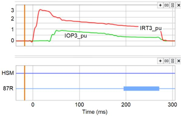
Fig. 23. Single Transformer Energization With HSM Disabled
