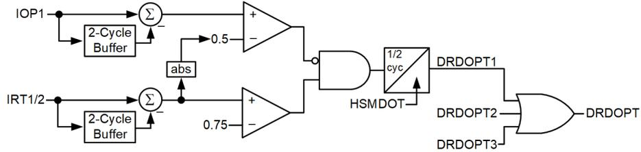
Fig. 9. Incremental Comparator External Event Detector
