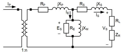
Fig. 1. CT Equivalent Circuit Referred to the Secondary Winding
