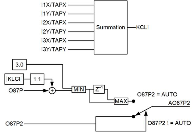
Fig. 11. Adaptive HSM Minimum Restraint Pickup Logic
