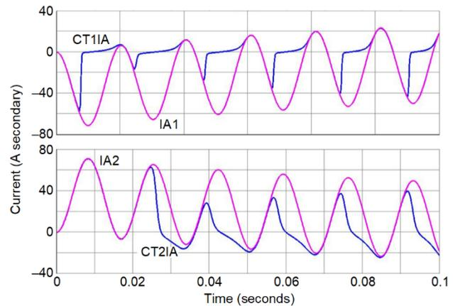
Fig. 20. Waveforms From an External Single Line-to-Ground Fault
