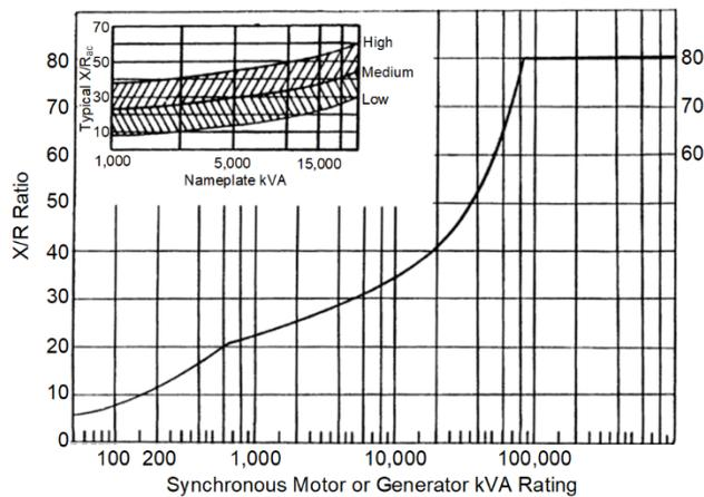
Fig. 28. IEEE X/R Ratios for Synchronous Machines [15]
