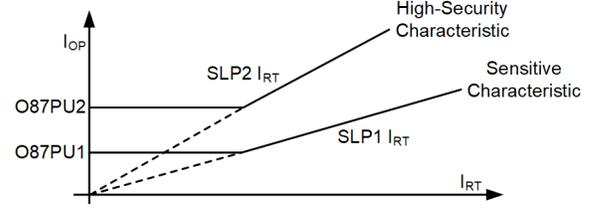
Fig. 6. Percentage Restraint Differential With HSM
