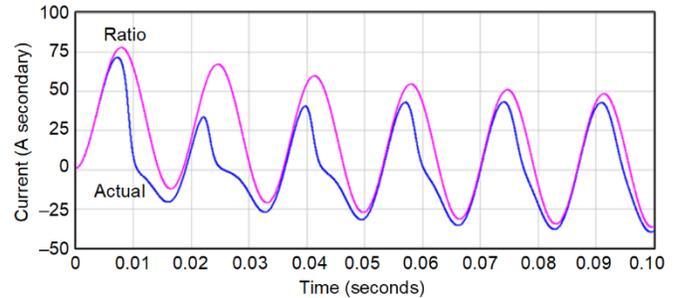
Fig. 18. Terminal CTs: CT2 Ratio and Actual Secondary Current
