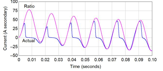
Fig. 17. Neutral CTs: CT1 Ratio and Actual Secondary Current
