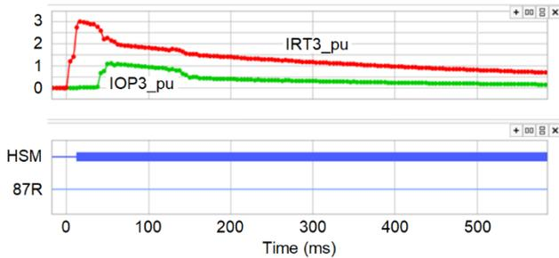
Fig. 24. Single Transformer Energization With HSM Enabled
