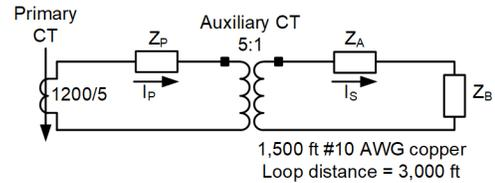
Fig. 5. Auxiliary CT to Reduce Apparent Leads Burden
