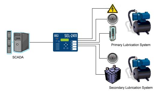
Figure 1 Backup Lubrication Monitoring and Control With Primary System Monitoring and Failover
