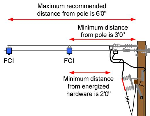
Figure 4 Placement of FCIs on Overhead Lines
