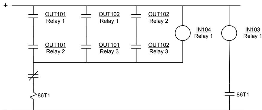
Figure 3 Tripping Channel 86T1
