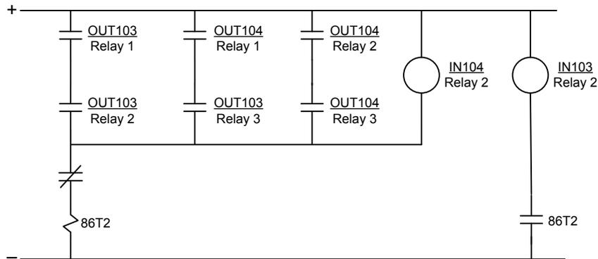
Figure 5 Tripping Channel 86T2
