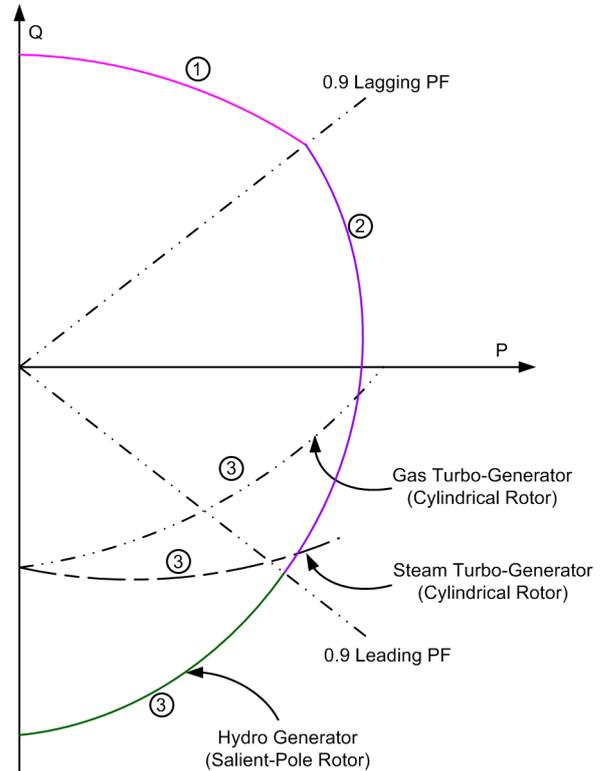
Fig. 2. GCCs for cylindrical-rotor and salient-pole-rotor generators.
