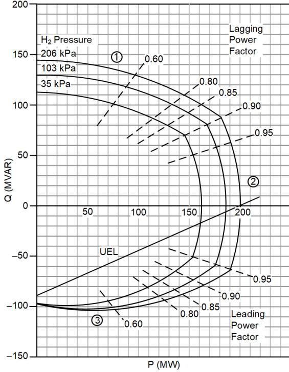
Fig. 3. GCC at nominal voltage of a 202 MVA, 15 kV, 0.9 pf, 3600 rpm, 60 Hz, hydrogen-cooled steam-turbine generator for various hydrogen pressures.
