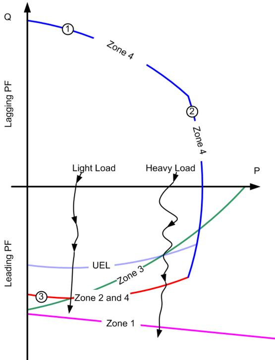
Fig. 4. P-Q-based LOF function with four zones.
