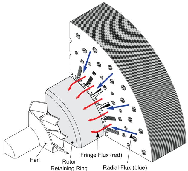
Fig. 1. The fringe flux (shown in red) between the stator-end-core region and the retaining ring increases when the rotor retaining ring comes out of saturation.
