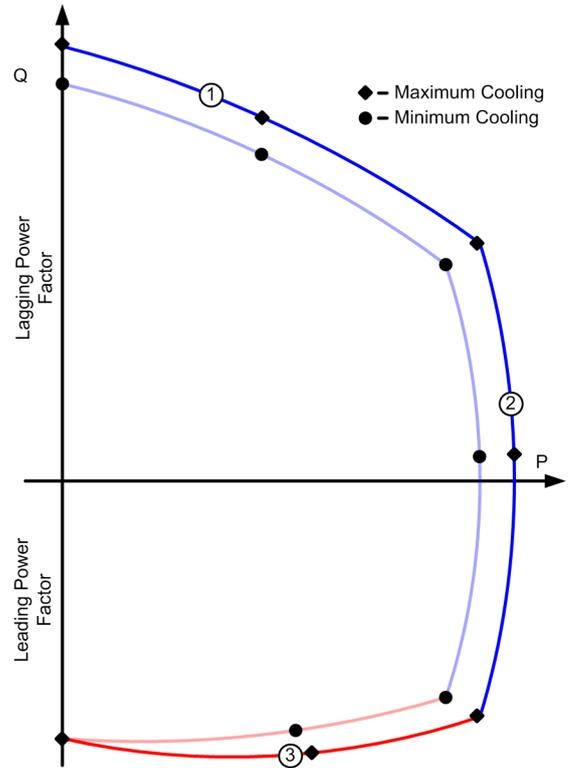
Fig. 5. Adaptive GCC replica based on cooling capability.
