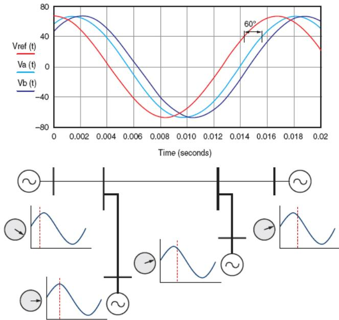
Fig. 6. Synchrophasor Measurement
