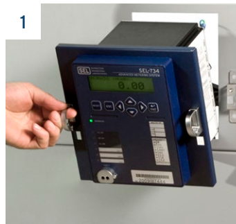
1 Pull quick-release latches.
