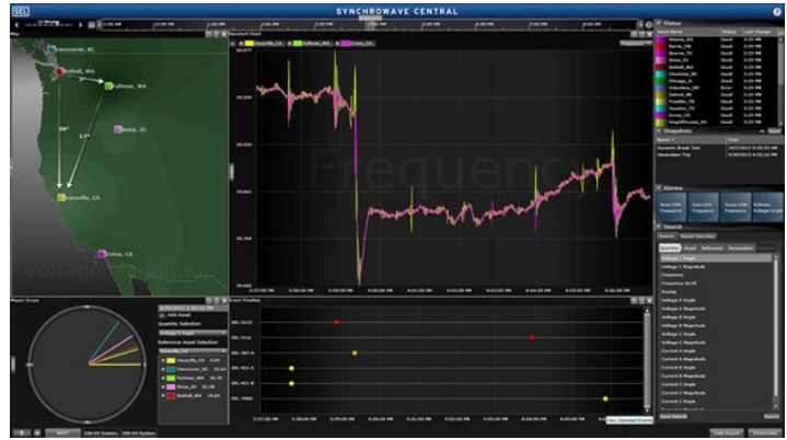
Monitor grid conditions with time-aligned synchrophasor messages.
