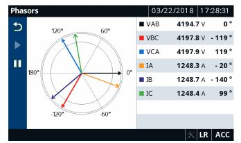
Figure 6 The Phasor application mimics a typical PC software view.
