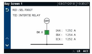
Figure 3 SEL Bay Screen one-line diagram with real-time status indication.
