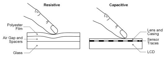
Figure 1 Touchscreen internal structures.
