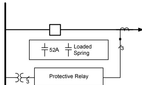
Fig. 4. Basic connection diagram for monitoring of circuit breakers
