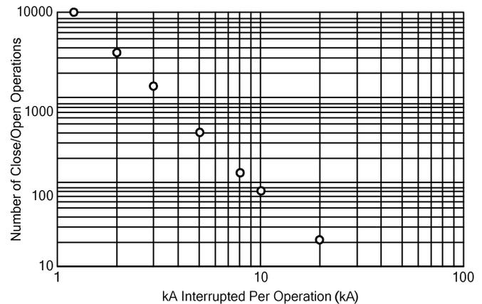
Fig. 3. Circuit breaker maintenance curve
