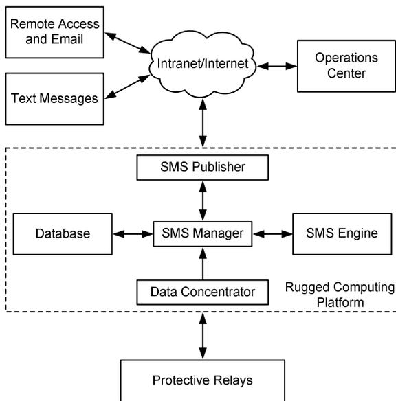
Fig. 12. Basic data structure of SMS
