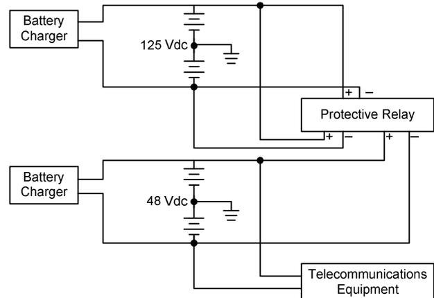
Fig. 6. Basic connection diagram for monitoring of two dc battery systems
