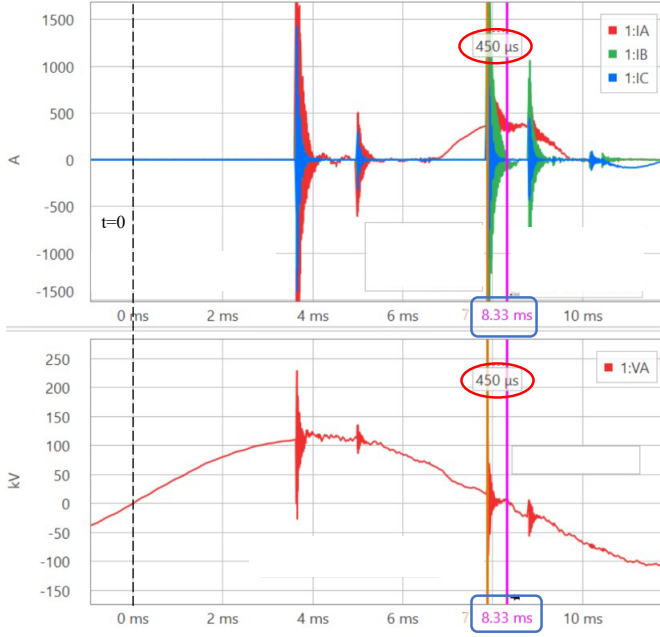
Fig. 20. Currents of Phases B and C and Reference VA for Case 5.
