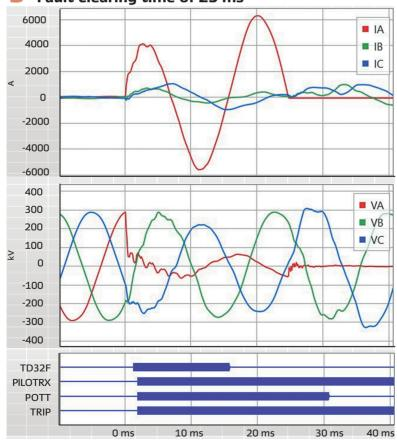
The TD32 element is fully independent on the fault point on wave and does not have any blind spots.
