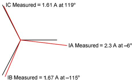
Fig. 4. In-service load readings
