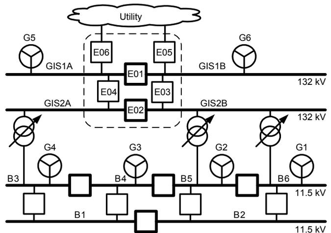
Fig. 1. Simplified one-line diagram of refinery power system [2].
