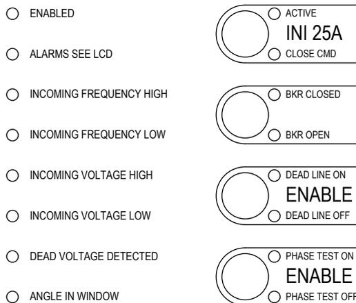
Fig. 5. Portable synchronizer controls and indications.
