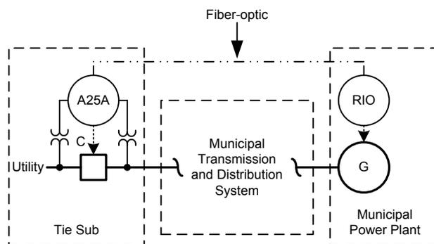
Fig. 3. Municipal microgrid with remote synchronizing.
