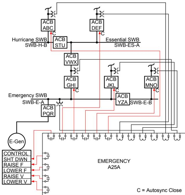
Fig. 2. Emergency generator A25A [5].
