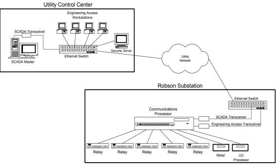
Figure 11 Robson Substation's New Integrated Communications With the Existing SCADA Master
