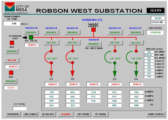
Figure 10 Robson SCADA HMI Display Using the New Communications Processor as the Data Source
