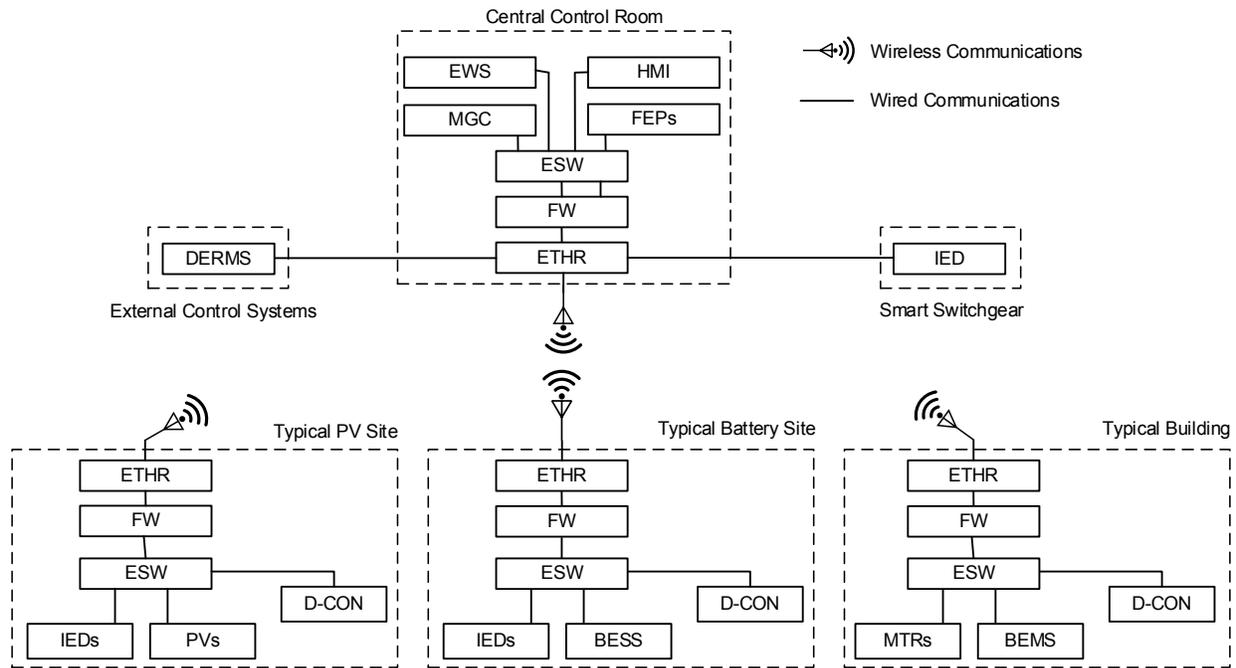
Fig. 4. Overall MGCS network architecture
