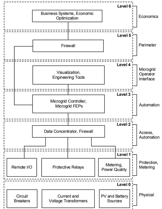
Fig. 3. Segmented MGCS architecture
