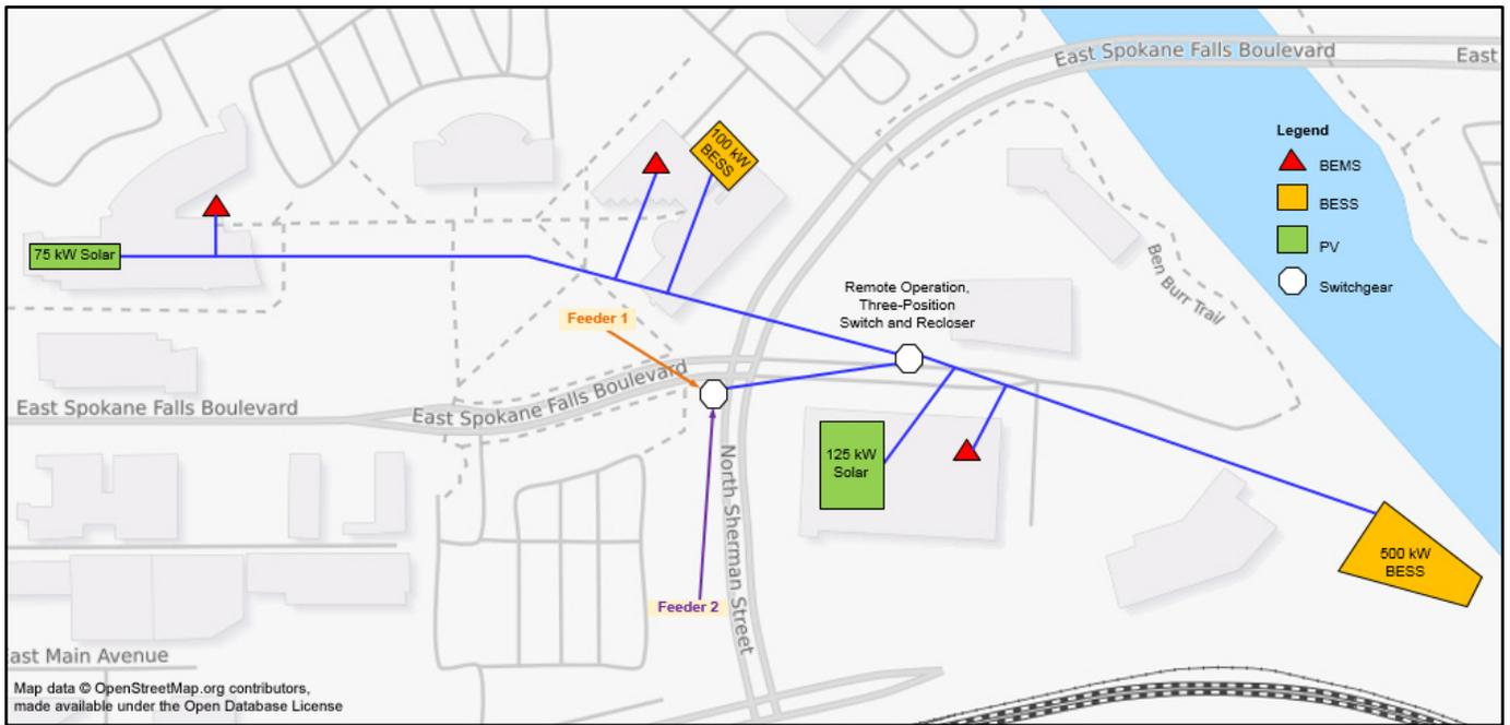
Fig. 1. Microgrid power system overview map
