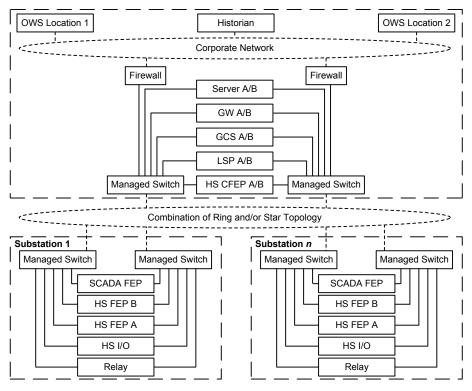
Fig. 2 Communications Architecture of the Oil Field
