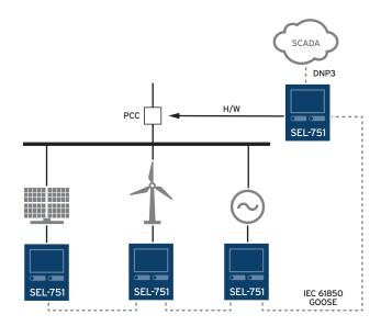
SEL relays at every power source provide system reconnection, load shedding, protection, IEEE compliance, power and power factor control, load sharing, dispatch, decoupling, synchronization, and frequency and voltage regulation.
