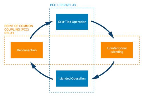
SEL relay-based microgrid systems provide seamless controls between all host-nation (grid-tied) power and islanded modes of operation.
