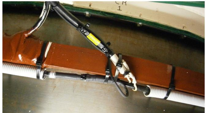
Fig. 22. A Rogowski coil with a test winding.
