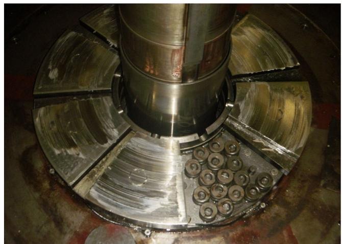
Fig. 16. Thrust bearing damage due to shaft currents (see striations in the bearing).
