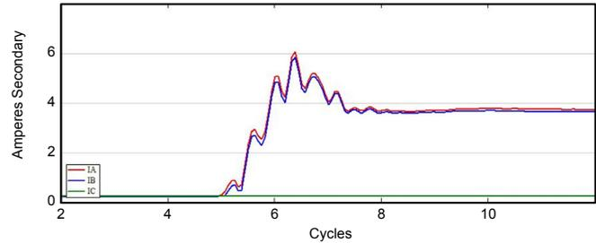
Fig. 26. Differential current magnitude for all phases.
