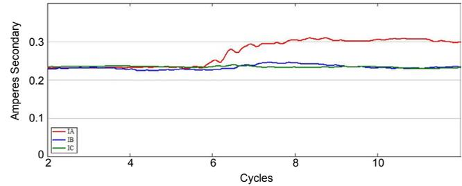
Fig. 38. Adjacent line A-phase single-line-to-ground fault.
