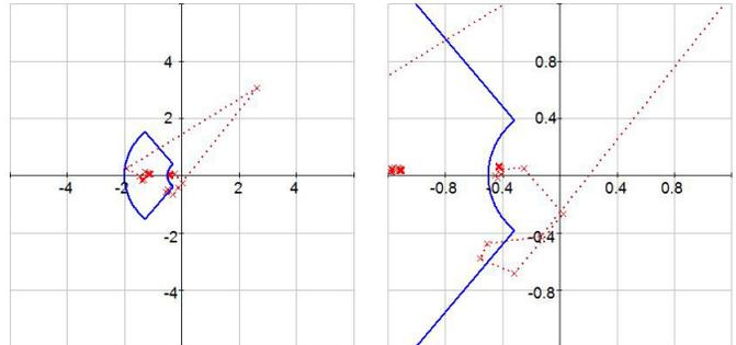
Fig. 47. Adjacent line A-phase-to-B-phase double-line-to-ground fault.
