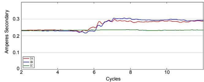
Fig. 40. Adjacent line A-phase-to-B-phase line-to-line fault.
