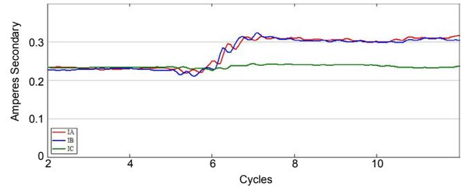
Fig. 39. Adjacent line A-phase-to-B-phase double-line-to-ground fault.
