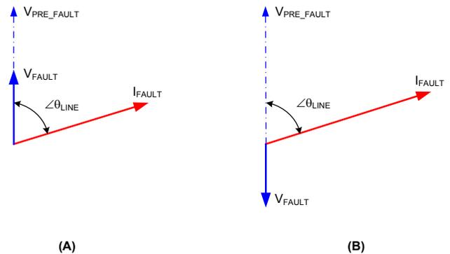
Fig. 8. Phasor relationship between the faulted phase voltage and current at Bus S when (A) the series capacitor bank is out of service and (B) the series capacitor bank is in service.
