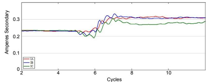
Fig. 41. Adjacent line three-line-to-ground fault.
