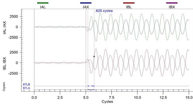
Fig. 30. Relay operation with reduced blocking angle.
