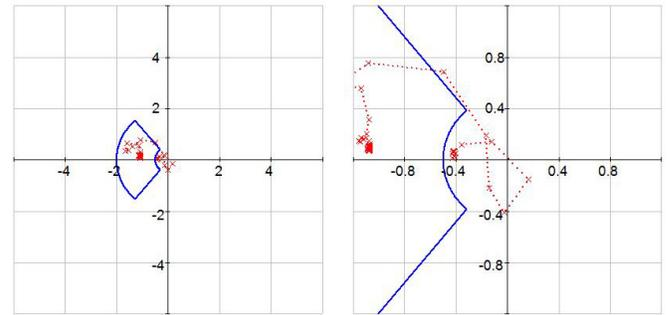
Fig. 48. Adjacent line A-phase-to-B-phase line-to-line fault.
