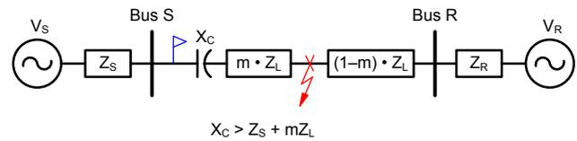
Fig. 10. Sketch of a simple power system in which current inversion can occur.
