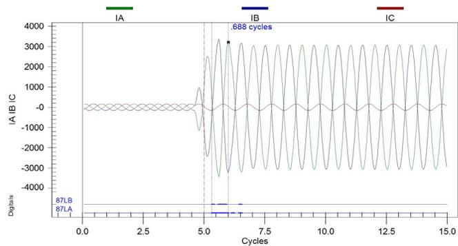
Fig. 32. Relay operation with reduced blocking radius.
