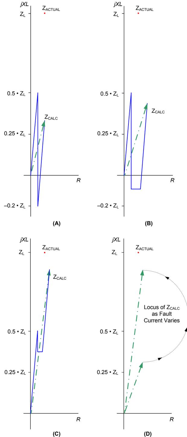
Fig. 5. Plots of the impedance calculated by the distance element for faults at the end of the line for varying values of fault current: (A) fault current is below the rated current of the series capacitor, (B) fault current is approximately 1.5–2.0 pu of rated current, (C) fault current is 6–7 pu of rated current, and (D) locus of impedance calculation for variation of fault current.
