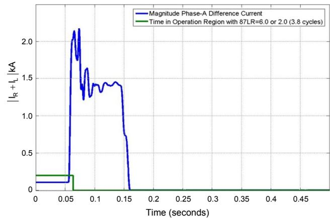
Fig. 22. Substation A difference current for initial transient analysis of a line-to-line fault for case study two.
