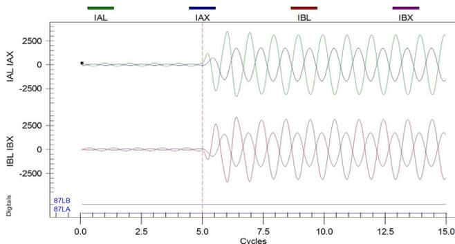
Fig. 25. Faulted phase currents for the line-to-line fault.
