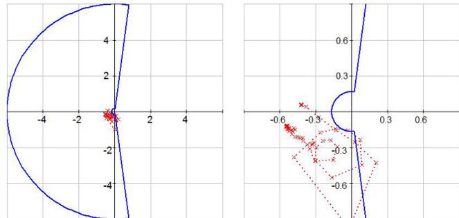
Fig. 27. A-phase alpha plane during the fault.
