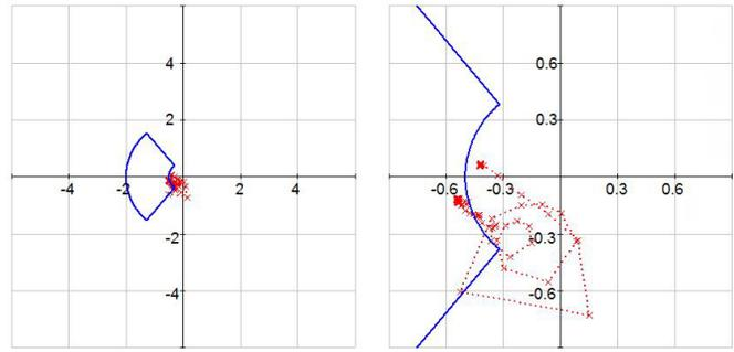
Fig. 31. Alpha plane with reduced blocking radius.
