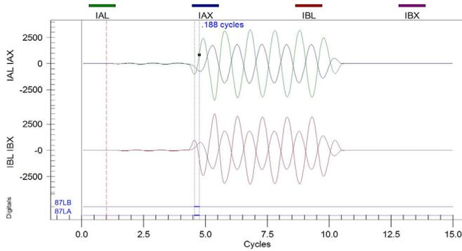
Fig. 28. Relay operation with reduced differential pickup.
