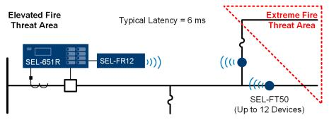
Figure 7 Dynamic Reclosing Application Using the SEL-FT50 and SEL-FR12
