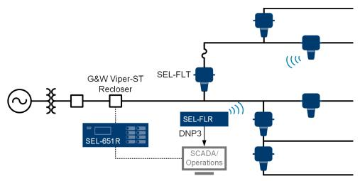
Figure 5 Example SEL-FLT and SEL-FLR Application
