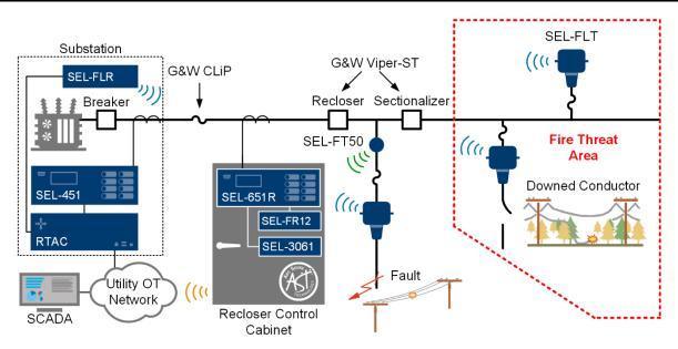
Figure 14 Fire Mitigation System Applications
