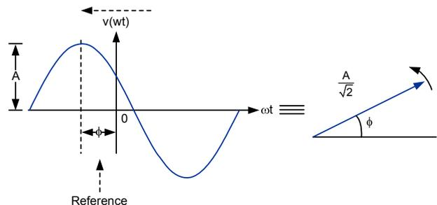
Fig. 2. Sinusoidal Voltage Time Waveform and Phasor Presentation
