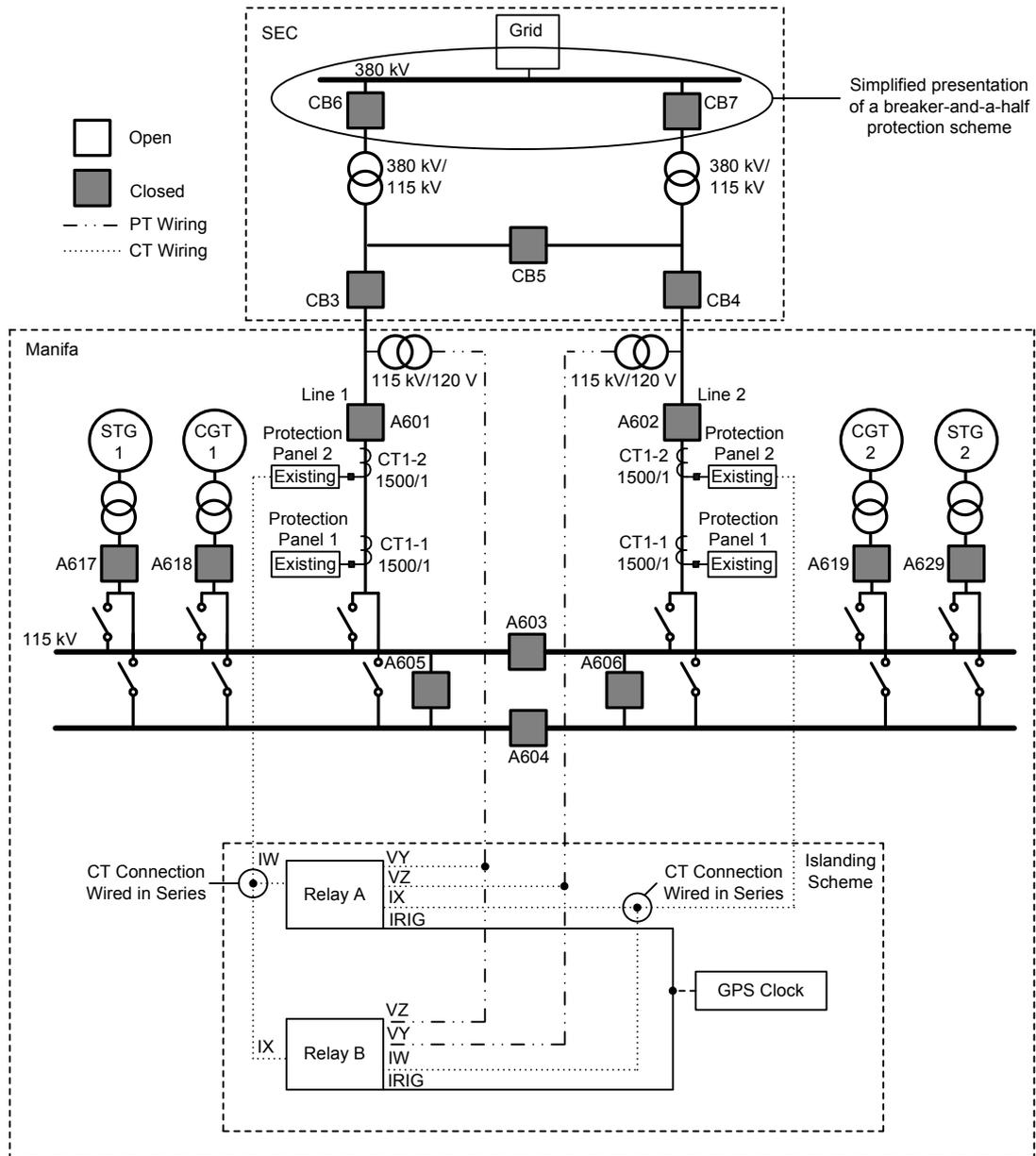
Fig. 1. Manifa System One-Line Diagram
