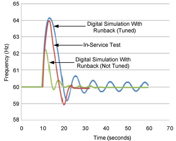
Fig. 11. Islanding CGT 1 Generator Runback Comparison
