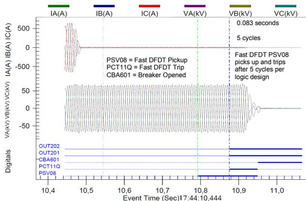
Fig. 10. Fast DFDT Operation for Remote-End Breaker Open
