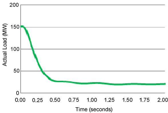
Fig. 9. Generator Runback During CGT 1 Islanding Test
