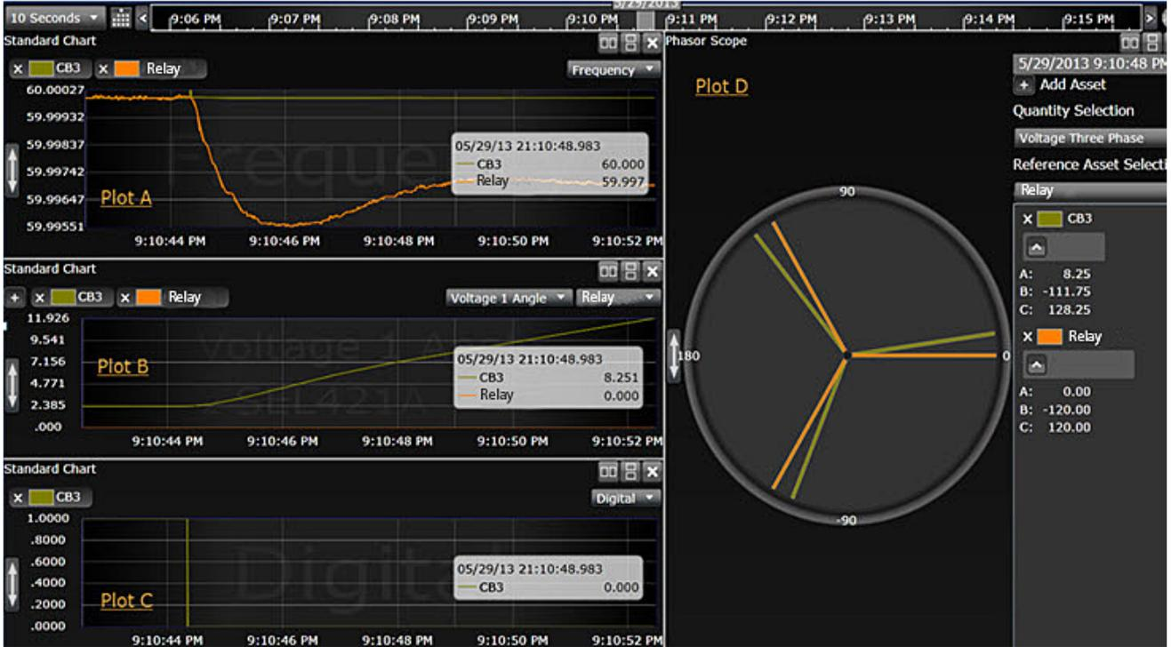
Fig. 7. Synchrophasor-Based Visualization (Phase Angle)
