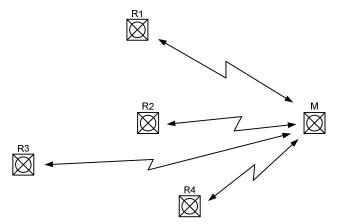
Figure 5. Point-to-multipoint radio application
