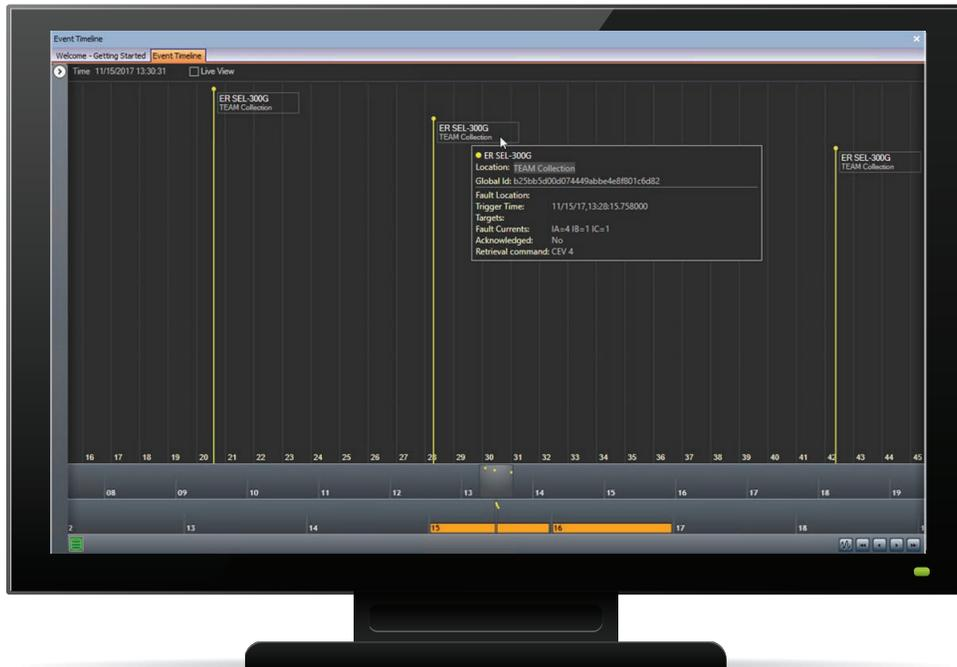
Quickly identify events using the Event Timeline viewer in acSELERATOR TEAM® SEL-5045 Software. You can hover over the flags to find the fault trigger time and fault currents.
