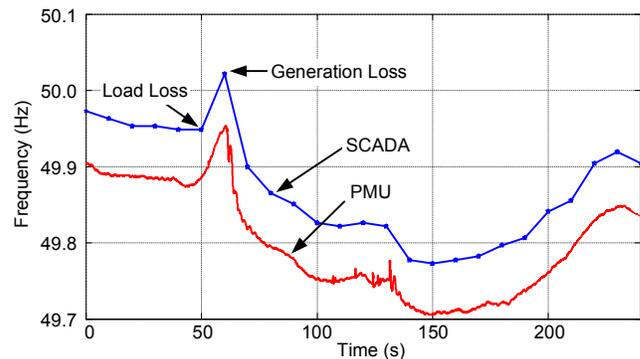
Fig. 10. Frequency measurements from SCADA have 70 mHz offset error
