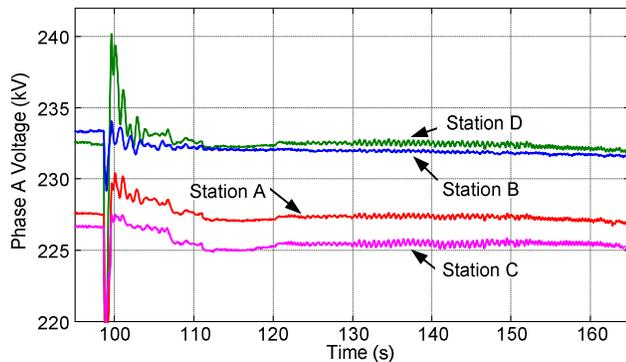
Fig. 12. Phase A voltage magnitude from synchrophasors
