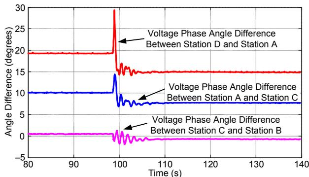
Fig. 15. Angle difference between Station D and Station A is greatest compared to the angle difference across other stations
