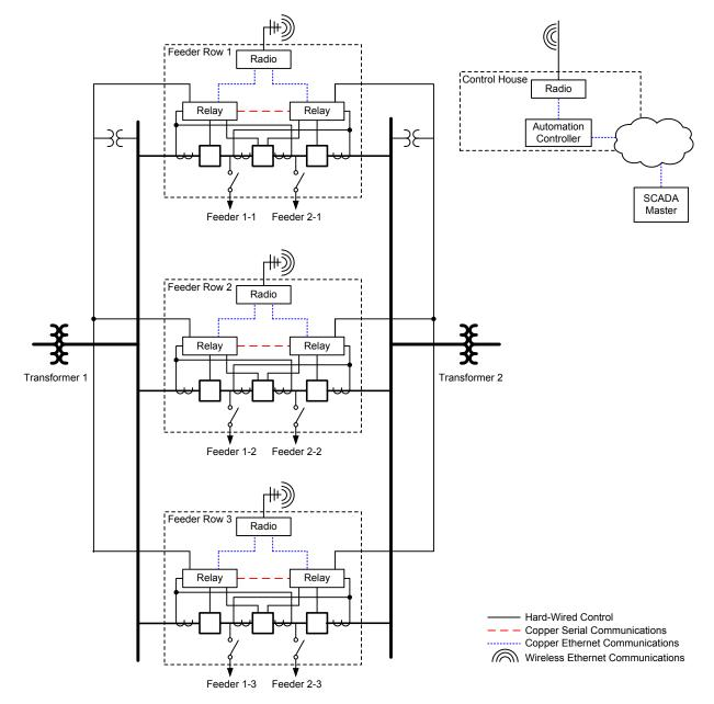
Fig. 2. Schematic of Three Communications Links to Three Feeder Rows in a Substation Yard
