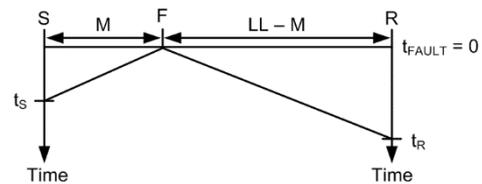
Fig. 6. Bewley diagram for a line fault.
