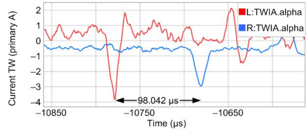
Fig. 3. Current TWs 10 ms before the fault.
