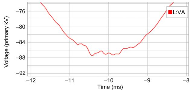
Fig. 4. Local Phase A voltage 10 ms before the fault.
