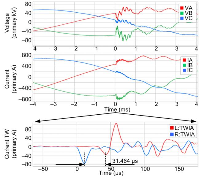
Fig. 11. Local voltages and currents, and local and remote current TWs (1 MHz record) for a 69 kV pilot installation.
