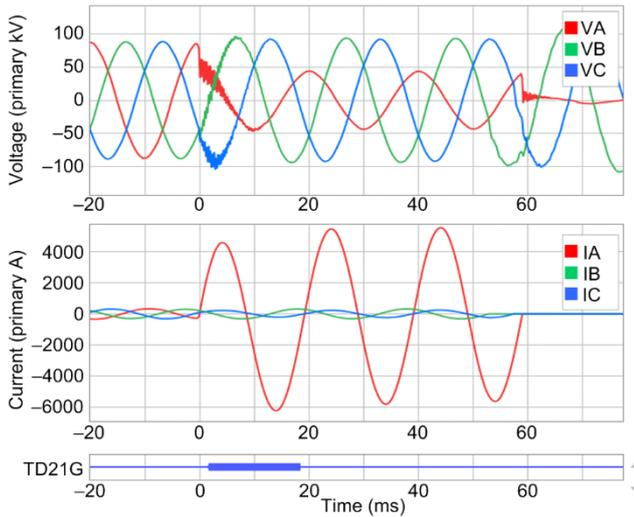
Fig. 1. Voltages and currents for an AG fault.
