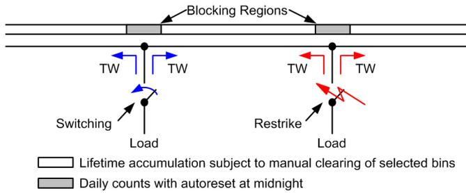
Fig. 9. Blocking regions for accommodating switching events at taps and series capacitors.
