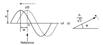
Fig. 1. Sinusoidal waveform translated to phasor representation
