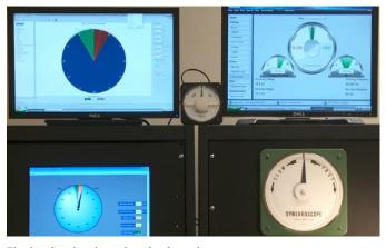
Fig. 3. Synchrophasor-based soft synchroscope test
