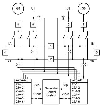
Fig. 6. Complex redundant automatic synchronizing system
