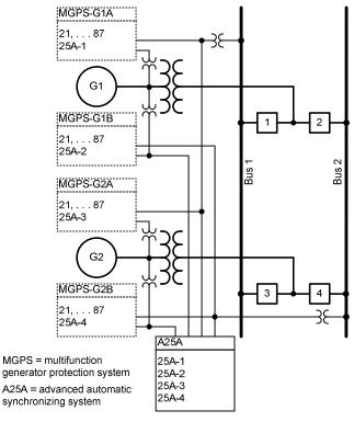
Fig. 4. Example applications using microprocessor-based automatic synchronizer(s) to eliminate VT signal switching
