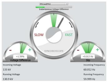
Fig. 2. Advanced PDC synchroscope
